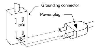
Connect the LABO-STIRRER's power plug to a receptacle with grounding connectors.
