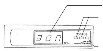
Revolving Speed Display (Ex: 300rpm)
