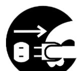
Compulsion, disconnect the power plug
