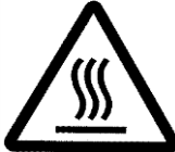
Warning, high temperature
