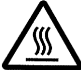
Warning, high temperature
