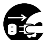
Compulsion, disconnect the power plug
