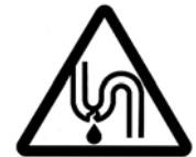
Caution for water leak!
