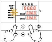
① Press the TIMER key on the initial screen. Press the TIMER key again. The setting temperature display screen displays the character "Astr", which indicates the auto start operation, with blinking.
