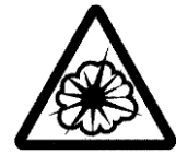
Danger!: Explosion Hazard
