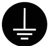
Connect grounding wire
