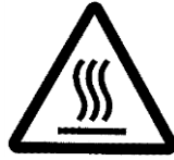
Danger!: High Temperature
