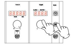
Turn the temperature setting dial clockwise to confirm that the temperature display is turned "on."
