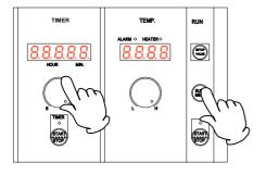
Start operation at the target set temperature and confirm the temperature in the bath with a temperature recorder after temperature has stabilized.
