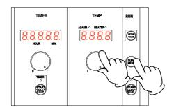
Turn the temperature setting dial anti-clockwise to confirm that the temperature display is turned "off."
