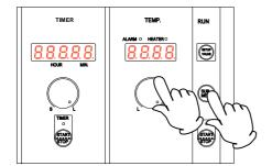
Turn the temperature setting dial to enter difference between the set temperature and the bath temperature. Turning the temperature setting dial clockwise increases setting and turning it anti-clockwise decreases it.
