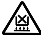
Caution: Do Not Heat Without Water!
