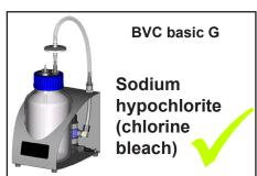
Aggressive disinfectants which release chlorine or oxygen radicals, e.g., sodium hypochlorite (chlorine bleach) or peroxide compounds can corrode the material of the 4l polypropylene collecting bottle and other components (e. g., couplings). This may lead to stress cracks and breakage of the 4l polypropylene bottle.
