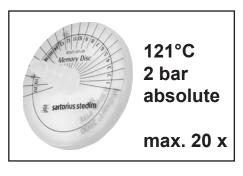
The number of autoclaving cycles can be marked on the plastic disc (Memory Disc) of the filter (max. 20 autoclaving cycles according to the manufacturer instruction).
