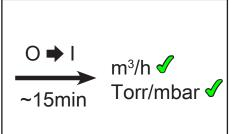
A warm up period (approximately 15 min.) is required to ensure that the rated ultimate vacuum and pumping speed are attained.
