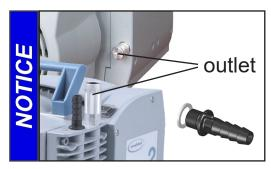
**Attention**: Use the (optional) silencer only in case of low gas throughput. Check the silencer regularly for permeability! In case, install a hose nozzle with sealing ring instead (see "Accessories", pg. 53).
