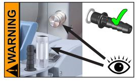
Operation with (optional) silencer at the outlet: Operating the pump at a high inlet pressure or pumping dusty gases for a long time may cause clogging of the (optional) silencer. Check the silencer regularly and replace if necessary, or install a hose nozzle with sealing ring instead (see "Accessories", pg. 53).
