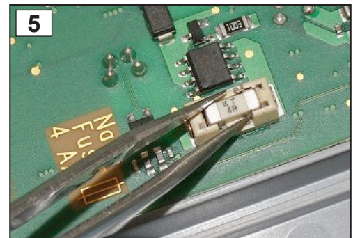
5. Insert the new fuse in the base.
