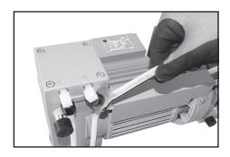
→ Loosen the union nuts of the hose connections at the pump head with an open-ended wrench (17 mm).
