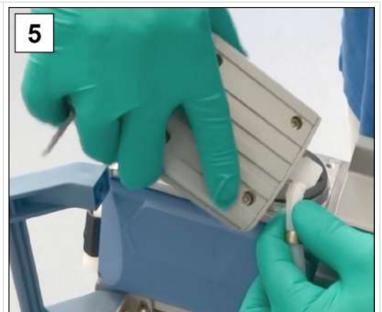
5. Once all valves are positioned correctly, initially insert the molded hose.
