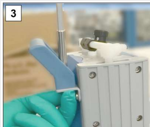
3. Loosen the screw fitting on the handle; hex key size 5.
