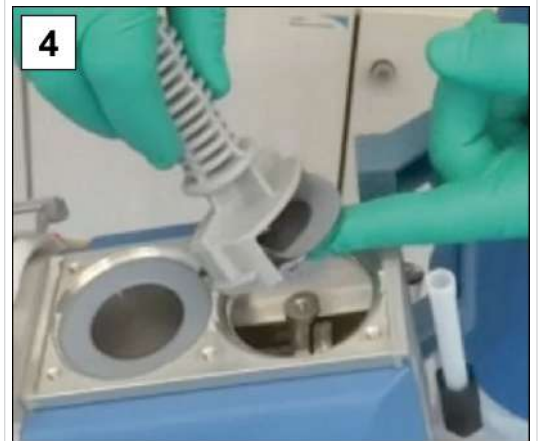
4. Lift the diaphragm, along with all the parts, out of the vacuum pump.
