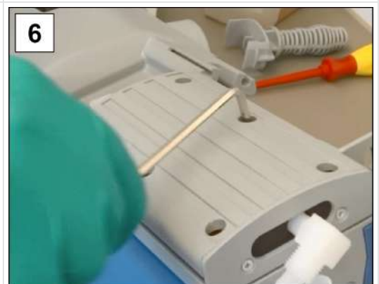
6. Unscrew the screw fittings; hex key size 4.
