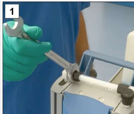
1. Loosen the union nut; open-end wrench SW17.
