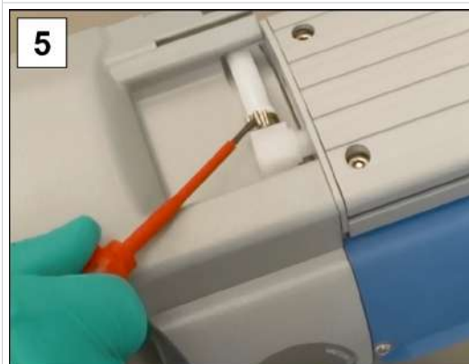
5. Open the hose clip; flat-head screwdriver size 1.
