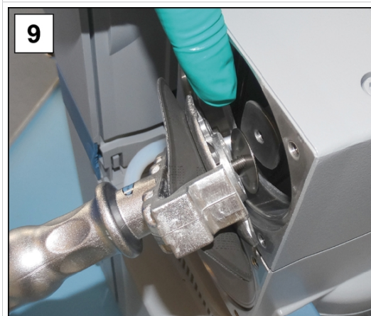
9. Hold onto the spacers and carefully place all components into the threaded hole of the connecting rod.
