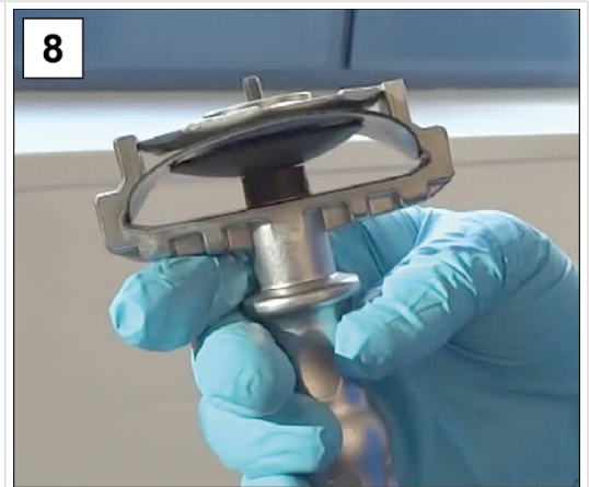
8. Attach the membrane assembly in the membrane wrench.
