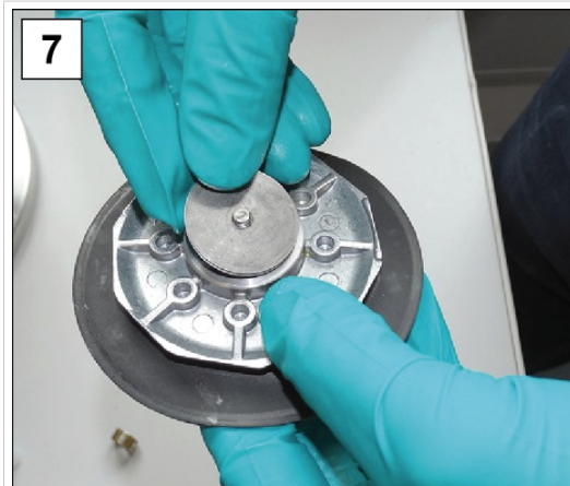
7. Place all spacers onto the threaded bolt.
