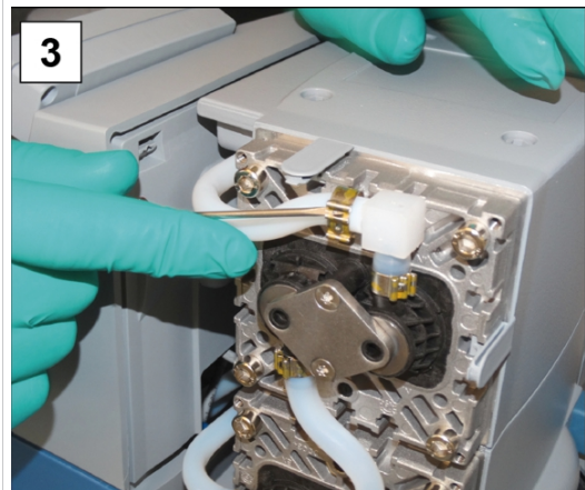
3. Open the hose clamps of the outer hoses. Flat-head screwdriver size 1.
