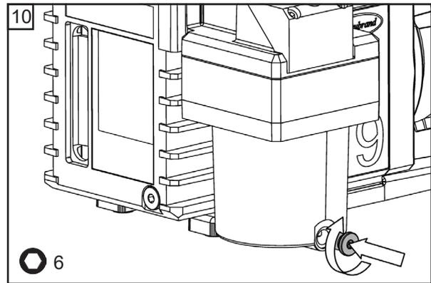
**Wechsel des Filterelements im Auspufffilter (20698008) / Replacing the filter element in the oil mist filter (20698008) RE / RZ 8 / 16 (20667077)**
