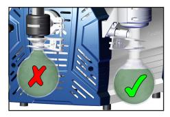
In case of **condensation**: Check the liquid level in the catchpots during operation. Check the liquid level in the catchpots regularly. Do not allow the catchpots to overfill. Drain catchpots in time to avoid overflow. Install a level sensor (see "Accessories / Spare parts", pg. 43) for monitoring, if necessary (VACUUBRAND controller CVC 3000 or VNC 2 is required).
