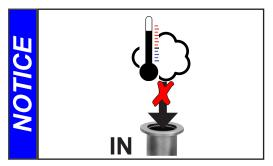
Avoid overheating (e.g., due to hot process gases). Maximum permissible temperature range: see "Gas inlet temperatures", pg. 27.
