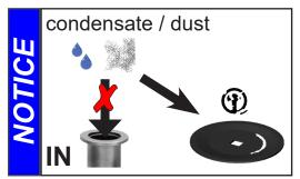
Prevent internal condensation, transfer of liquids or dust. The diaphragms and valves will be damaged, if liquids are pumped in significant amounts.
