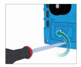
**1.** Use a Phillips screwdriver to unscrew the screw of the battery compartment lid.
