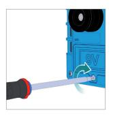
**4.** Put the battery compartment lid in correct position onto the gauge and fix it stress-free by the captive screw. When tightening, observe the maximum torque of 0.4 Nm.
