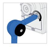
**2.** Turn the gauge into a suitable position and fix it with the counter nut of the support rod.
