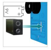
**3.** Put in the new battery in correct position (compare to figure inside the housing).
