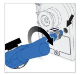
1. Screw in the support rod into the blind hole on the rear side.
