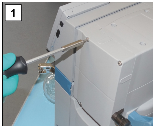
1. Undo the screw fasteners from the head cover; Torx screwdriver TX20.
