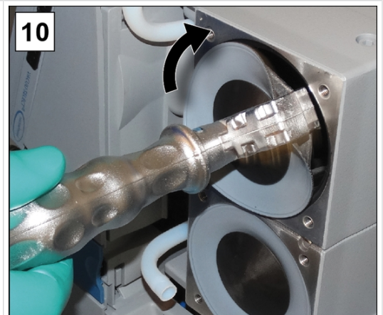
10. Tighten the assembly by hand at first using the membrane wrench.
