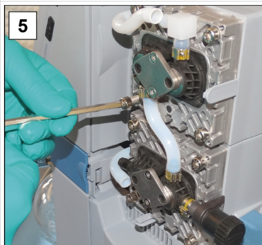
3. Open the hose clamps of the outer hoses. Flat-head screwdriver size 1.
