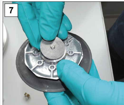
7. Place all spacers onto the threaded bolt.
