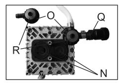
Remove valve heads (O) along with the disc springs (R), connection tube if applicable, hose nozzles (P) and connection fasteners (Q) or move the valve heads carefully aside. Note position and orientation of the valve heads.
