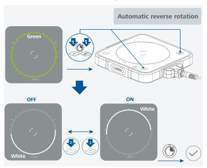
> Continue setting the interval time, after the reverse rotation function has been activated.
