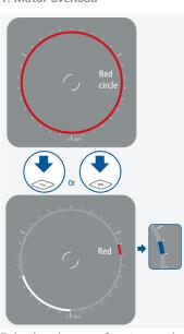
If the allowed motor power is overloaded by the user application, the device automatically reduces the speed value step by step until the motor can reach a stable operating state.
