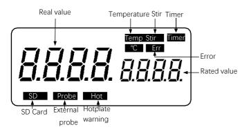
Figure 5 LCD digital model
