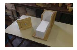
5. Open dry ice block machine by loosening latches and folding down sides. Remove block for use or storage. Caution: always wear protective gloves when handling dry ice; can cause burns and frostbite. Blocks can be stored in Dilvac Dewar Flasks. 6. During and after making dry ice block, handle feed hose carefully. Hose will appear white and is frozen. If bent, pulled or twisted hose can be damaged or broken.
