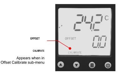
**To Access:** Press the **()** key until OFFSET CALIBRATE appears on the display.
