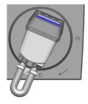
3. Lift the Controller straight up and out of the opening of the Circulator's top deck.
