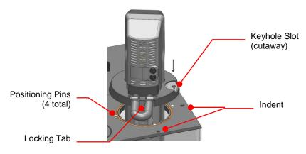
2. Gently rotate the Temperature Controller until it drops down on the Positioning Pins.
