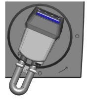
3. Rotate the Temperature Controller counterclockwise until the Locking Tab engages the indent on the top deck.
