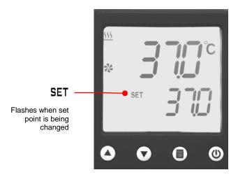
**To Change:** Press the or the key. The word "SET" will begin flashing. Continue holding or repeatedly press or the until the desired set point temperature is displayed.
