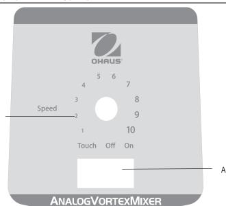
The front panel of the Analog Vortex Mixer contains all the switches and control knob needed to operate the unit.
