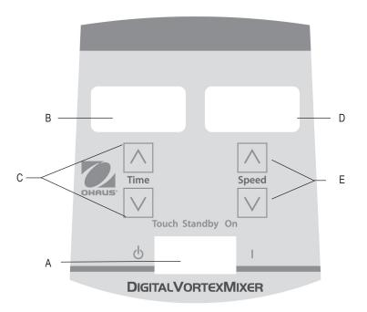
The front panel of the Digital Vortex Mixer contains all the switches, controls and displays needed to operate the unit.
