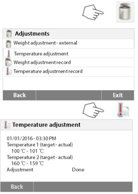
Press Weight and temperature adjustment button to access the adjustment screen. Press **Back** to return to previous screen. Press **Exit** to return to Home screen. Press the Temperature adjustment history button.
