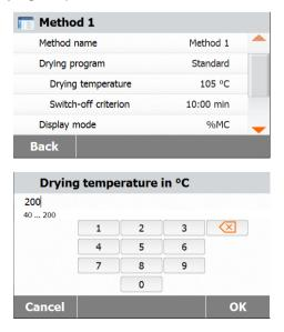
Press the Drying Temperature button to access the temperature setting menu.
