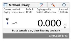
The analyzer comes with a default method preinstalled. Follow the instruction message to start a measurement directly. Press parameters area to edit.
