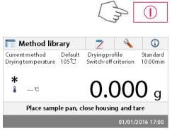
To **switch the Moisture Analyzer on**, press the **On/Off** button. An internal diagnostic test is performed; the display lights and the Home screen appears followed by the initial display.
