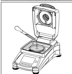
Place the empty sample pan and glass fiber pan in the pan handle. The sample pan must lie flat in the pan handle.
