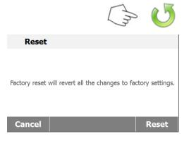
Press Factory reset button to reset to factory default settings.
