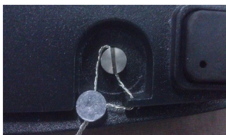
Locked with Wire Seal
