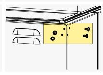
3. Attach the mounting bracket to the lid and fix in place with the screws.
