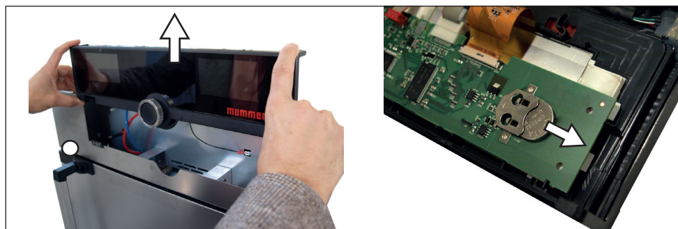
Fig. 30 Removing the lithium battery
