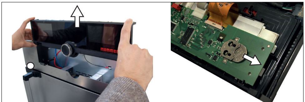
Fig. 25 Removing the lithium battery
