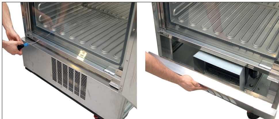
Fig. 25 Unscrew and remove the front cover
