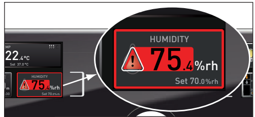
Fig. 22 Humidity monitoring triggered
