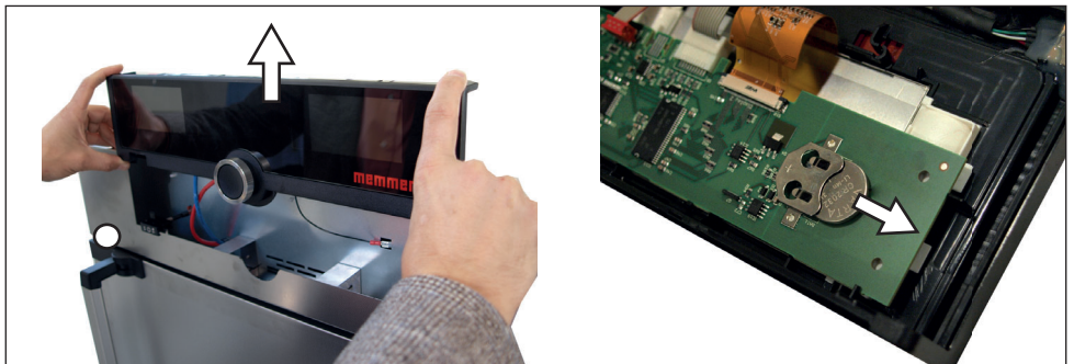
Fig. 34 Removing the lithium battery
