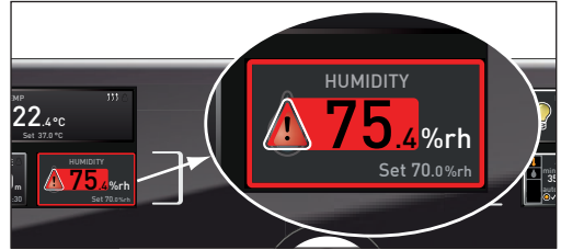
Fig. 22 Humidity monitoring triggered
