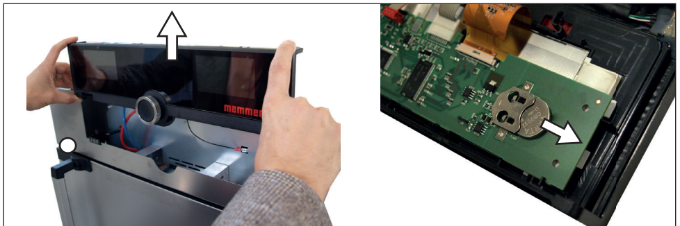
Fig. 29 Removing the lithium battery
