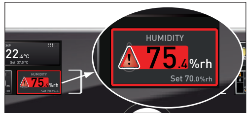
Fig. 21 Humidity monitoring triggered
