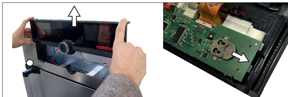
Fig. 25 Removing the lithium battery
