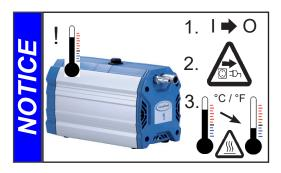
In case of overload, the motor is shut down by a **self-hold thermal cutout** in the winding. **Note**: Only manual reset is possible. Switch off the pump and disconnect from the power source. Identify and eliminate the cause of failure. Allow the pump to cool down sufficiently before restart
