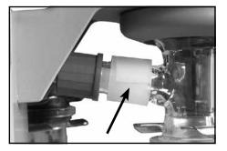
Overpressure safety relief device ......**20638821** (at exhaust waste vapor condenser)
