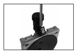
Loosen connection fastener slightly.
