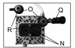
Remove valve heads (O) along with the disc springs (R), connection tube if applicable, hose nozzles (P) and connection fasteners (Q) or move the valve heads carefully aside. Note position and orientation of the valve heads.
