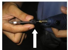
Put collette onto the shaft and screw it back to the drive itself! While doing that you must press the black button to lock it
