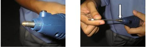
Remove collette and insert axle of the shaft into its place!
