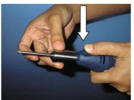
Press the black locking button and screw it fully onto the drive!
