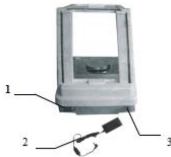
1. Data Interface 2. Transformer 3. Electrical Outlet
