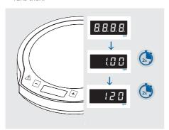
> Touch "+" to increase the speed, "-" to lower the speed, and both of the keys to set the speed to "0".
