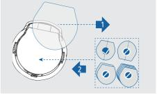
Assemble the stirring part back to the external part.
