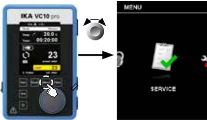
In the "Service" menu, the valves, the pump or the refrigerated circulator can be operated individually and also checked to ensure that they are operating correctly. If no VACSTAR is connected, the menu item "Pump" is greyed out and not active.
