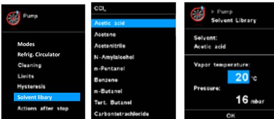
In the “solvent library”, the most common solvents are assigned a function to determine the steam temperature at the set pressure and vice versa. This provides assistance when setting these parameters in manual mode, for example, evaporation processes with a rotary evaporator.
