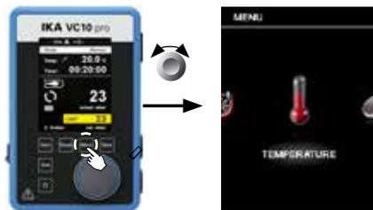
In the "Temperature" menu the user can specify that the temperature sensor is displayed on the display/working screen. A tick (✓) shows that the option is activated.
