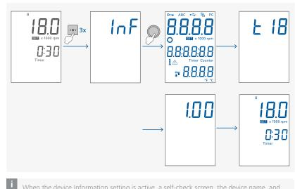
When the device Information setting is active, a self-check screen, the device name, and the software version will appear.
