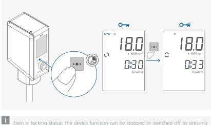
Even in locking status, the device function can be stopped or switched off by pressing the control knob (C) or standby button (D).
