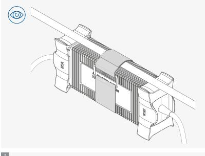
i If required, the desktop power supply can be attached to a horizontally aligned pole using the brackets and the holding band supplied.
