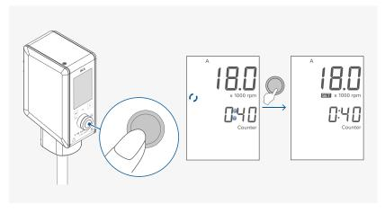
i > After stopping the device function, the last speed setting is shown on the display.
