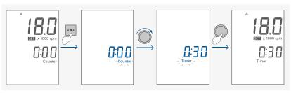
i > If the value of the timer/counter setting is set to 0:00, the counter function is activated and the corresponding symbol (Counter) lights up.
