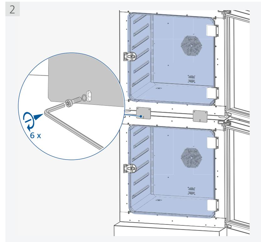
› Attach the upper device to the wall
