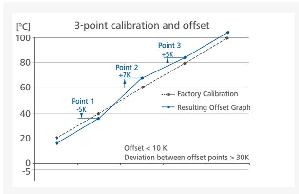
Individual load and ambient condition might influence the temperature behaviour of the chamber. To compensate that influence there's the option to neutralize by using the 3-point calibration and offset function. This function allows the temperature to be calibrated and adjusted at three different temperature values.
