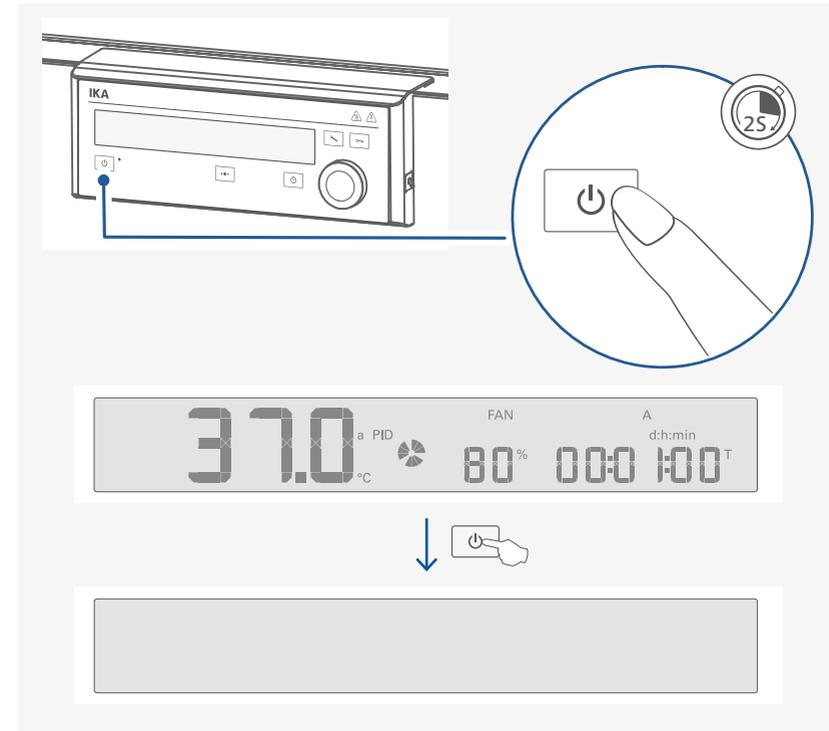
**Note:** When switching the device to standby status, if the device chamber temperature is higher than 50 °C, the actual temperature is displayed, e.g. 70 °C and "hot" symbol blinks.
