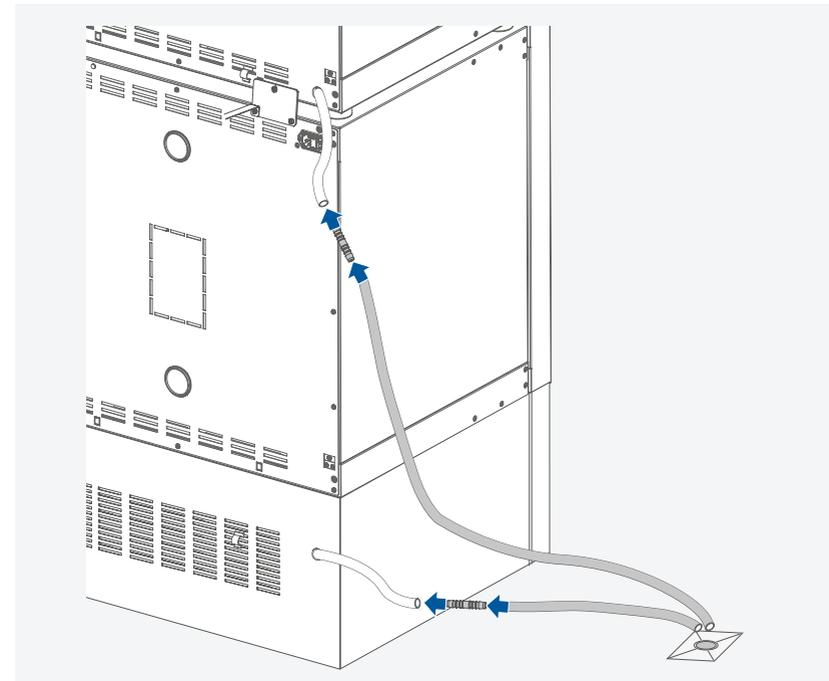
The devices drain hoses must be guided to the laboratory drain with the hose adapters and extension hoses.
