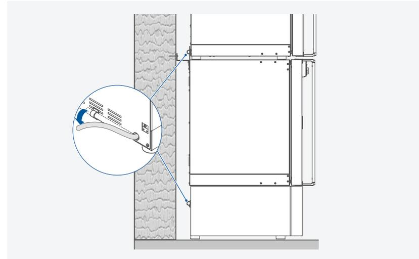
Extend the drain hose as required using the enclosed hose adapter
