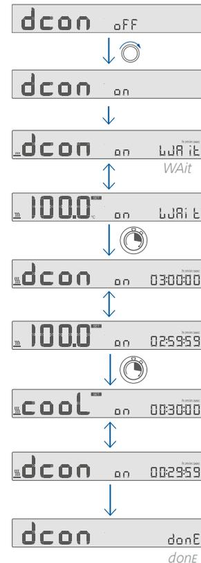
When the decontamination process is finished, the "dcon done" appear on the display and a "beep" sound is heard.
