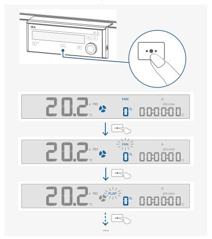
**Note:** Press the multifunction key (F) to switch between the settings for the fan and the ventilation flap. The selected function blinks. Then, the value can be adjusted respectively by rotating the control knob (H).
