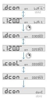
When the decontamination process is finished, the "dcon donE" appear on the display and a "beep" sound is heard.
