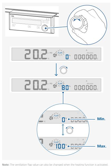
> Confirm the setting of the opening of the ventilation flap
