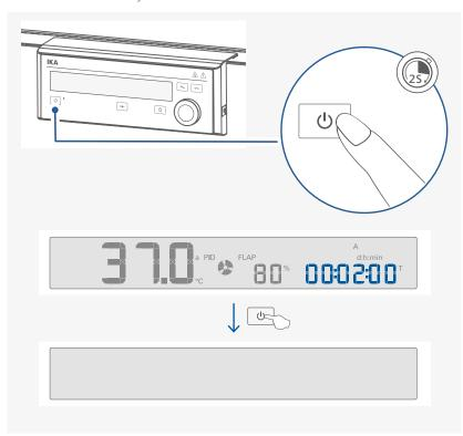
**Note:** When switching the device to standby status, if the device chamber temperature is higher than 50 °C, the actual temperature is displayed, e.g. 70 °C and "hot" symbol blinks.
