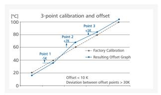
Individual load and ambient condition might influence the temperature behaviour of the chamber. To compensate that influence there's the option to neutralize by using the 3-point calibration and offset function. This function allows the temperature to be calibrated and adjusted at three different temperature values.
