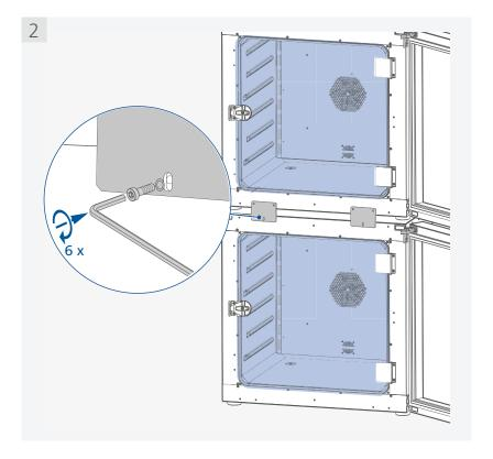
> Fix the top device to the wall
