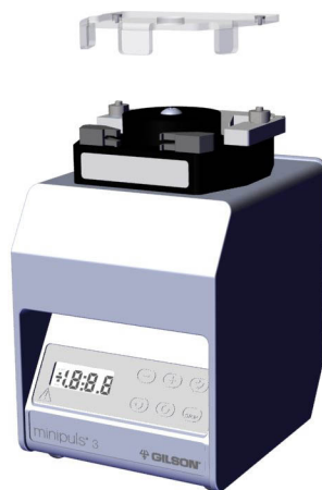
Figure 14 Safety Cover Installation
