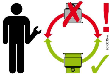
Figure 17 Mounting orientation for nEXT1230H
