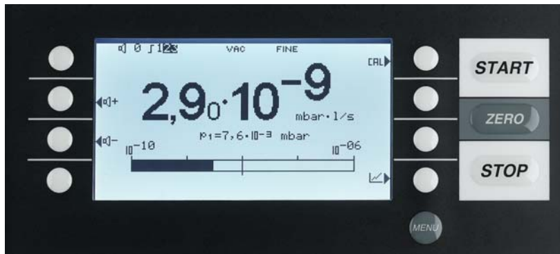
Figure 9 Display: measurement mode with bar graph
