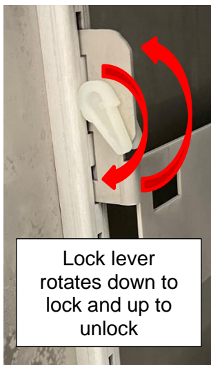
Drawer Bracket Lever Lock
