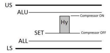
During the normal operation, the cabinet's compressor would turn on and off, to maintain the controlled room temperature in the storage chamber.
