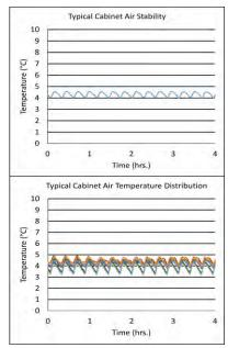
Performance data acquired at 22°C ambient, 4°C nominal set point in an empty cabinet with shelves using air probes, during stabilized steady state operation and a DAQ sampling rate of one measurement every 10 seconds
